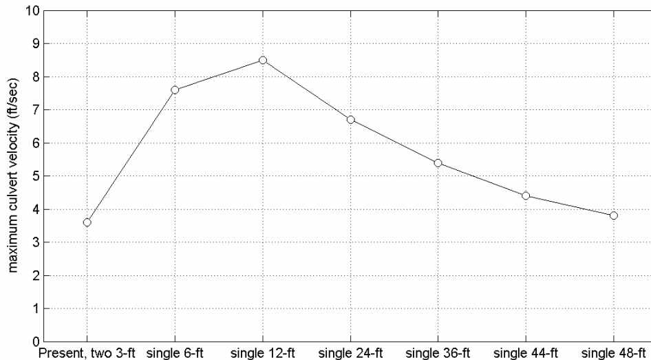
Figure 5. Maximum modeled culvert velocities for present conditions (two 3-foot culverts) and five single culvert scenarios for Muddy Creek.
